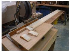
Some boards are checked (the grain is running the wrong way) and occasionally there is some waste. However, many car bodies can be salvaged with a bit of wood glue and a couple of rubber bands.
