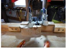
Unfortunately, after the axle holes are drilled, the car body needs to be sanded, especially the sides since they are end grain. Sanding with 80 or 100 grit paper is usually sufficient since
