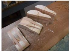
After the car bodies are cut, holes need to be drilled for the axle pegs. The pegs are ½" in diameter and the holes need to be sized to provide a tight (but not too tight) friction fit. Depending upon your drill bit collection, there are some options:
